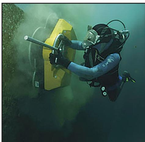
**Figure 3.1: Underwater hull cleaning with no capture system evident**
